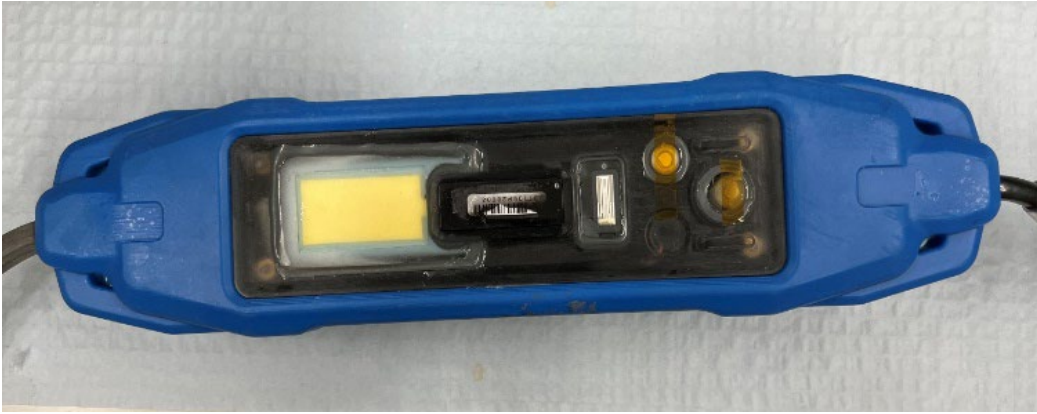
Figure 2: Vesit TM sensor pack using solid-state reference electrode with ORP, pH, conductivity, and temperature sensors.
