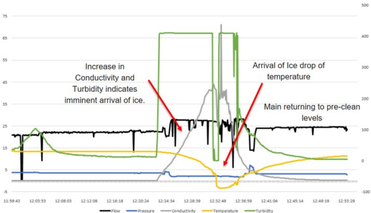
Figure 3: Parameters from discharge point during ice pigging operation (operation 18)
